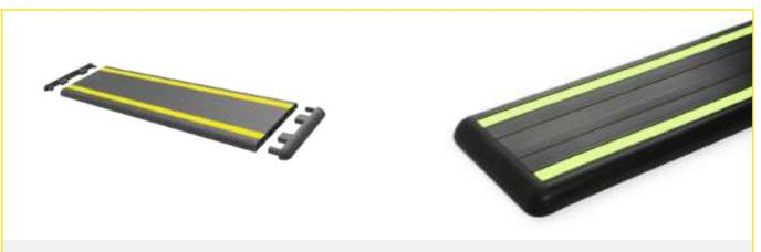
Rubber wall guard system with a width of 150 mm and a thickness of 20 mm is used in parking lots and factories or in areas where deformation can be more intense to prevent deformations that may occur on the walls. It creates a decorative appearance with its right and left end caps. Profile lengths are manufactured as 3 meters.
