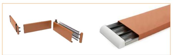
WG200 is a wall protection tape with a width of 200 mm and a depth of 35 mm, which is mounted on the wall with a continuous rear aluminium profile. It absorbs the impacts thanks to the lower Styles. Thanks to its 35 mm depth and lift shock absorber wick, it is used especially for heavy-duty corridors for protection against impacts. Profile lengths are 4 meters and are produced in 32 different colours.
