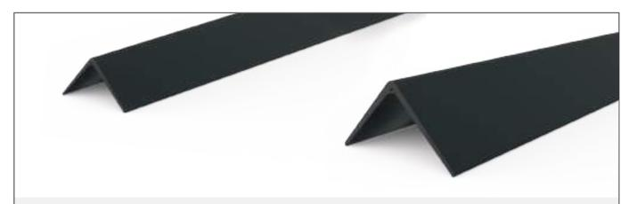
It is a TPE based corner protection profile which is applied with suitable adhesives to wall and column corners with width of 50 - 100mm wing. They are manufactured in 1000 /1500/3000 mm lengths.
