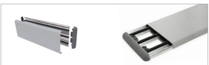
WG 201 is a wall protection tape with a width of 200 mm and a depth of 20 mm, which is mounted to the wall with a continuous rear aluminium profile. It absorbs the impacts thanks to the lower wicks. It provides a wide protection area in corridors narrower than 2 meters thanks to its 200 mm top width. For this reason, they are highly preferred in hospital corridors that are in intensive use. Profile lengths are 4 meters and are produced in 32 different colours.
