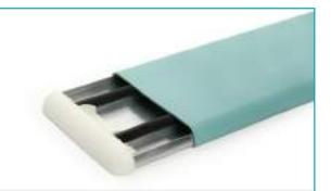
WG 150 is a wall protection tape that is mounted on the wall with a continuous aluminium profile with a width of 100 mm and a depth of 20 mm. It absorbs the impacts thanks to the bottom wick. They are used to protect the walls against impacts in areas where the use of wall protection tapes with hand grips is not appropriate, especially in corridors narrower than 2 meters. Profile lengths are produced in 4 meters.
