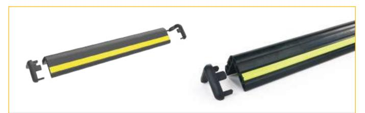
RG80 Rubber corner protection system is used both in parking lots and factories or in areas where deformation is more intense to prevent deformations in column and wall corners. It creates a decorative appearance with its top end caps. It can be used in a specific height (L: 1 m, L: 1.50 m) as well as throughout the floor height. Profile lengths are manufactured as 3 meters.
