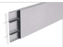
It is a stainless wall protection band formed by attaching a 200 mm wide 1.00 mm thick 304 quality stainless sheath to aluminium carrier profiles. It absorbs the impacts thanks to the shock-absorbing wicks.
