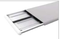
It is a door plinth band that is mounted on the lower part of the doors with a profile on aluminium with a width of 150 mm and a depth of 10 mm. It is produced with lower TPE to prevent the doors from being damaged in the passing traffic of heavy service cars. It is common in service corridors, swing doors, and elevators to dampen shocks. Profile lengths of 4 meters are produced.
